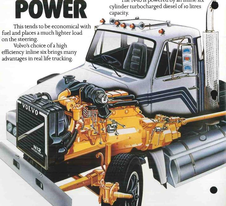
For durability all gears are induction hardened and driveshafts are heat treated.
