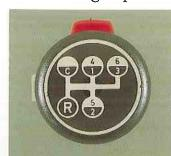
The gear lever showing how the SR-70 achieves 14 speeds with just three forward and one reverse positions.
