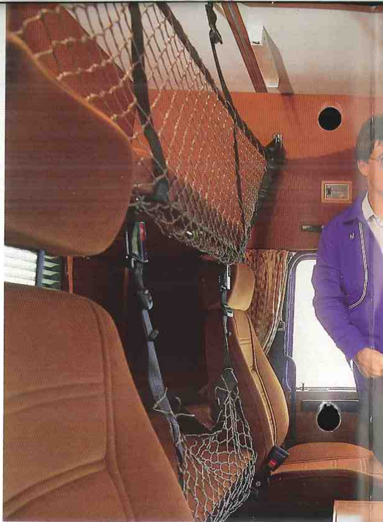
The high ceiling of the Globetrotter (370 mm higher than the regular F-Series cab) enables tall drivers to stand and change clothing.
